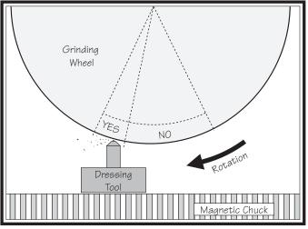
Figure 37. Safe tool positioning for wheel dressing.
